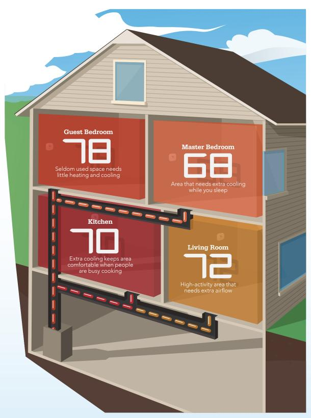
Airflow supply is varied to each zone throughout the house to meet a wide range of heating and cooling needs, while also reducing energy costs by up to 35%.\*
