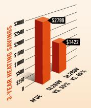
AFUE stands for "Annual Fuel Utilization Efficiency" and is a measure of a furnace's efficiency and performance. Like the milesper-gallon rating on your car, the higher the AFUE rating, the lower your fuel costs. Typical furnace ratings range from 80% to 95%.
